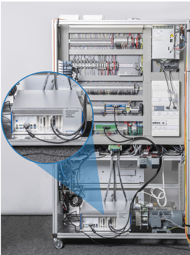
Top left: front view of the Controller HIL System Middle right: Manuel Pijorr, Senior Simulation Engineer Bottom right: back view of the Controller HIL System with the Performance real-time target machine in place
